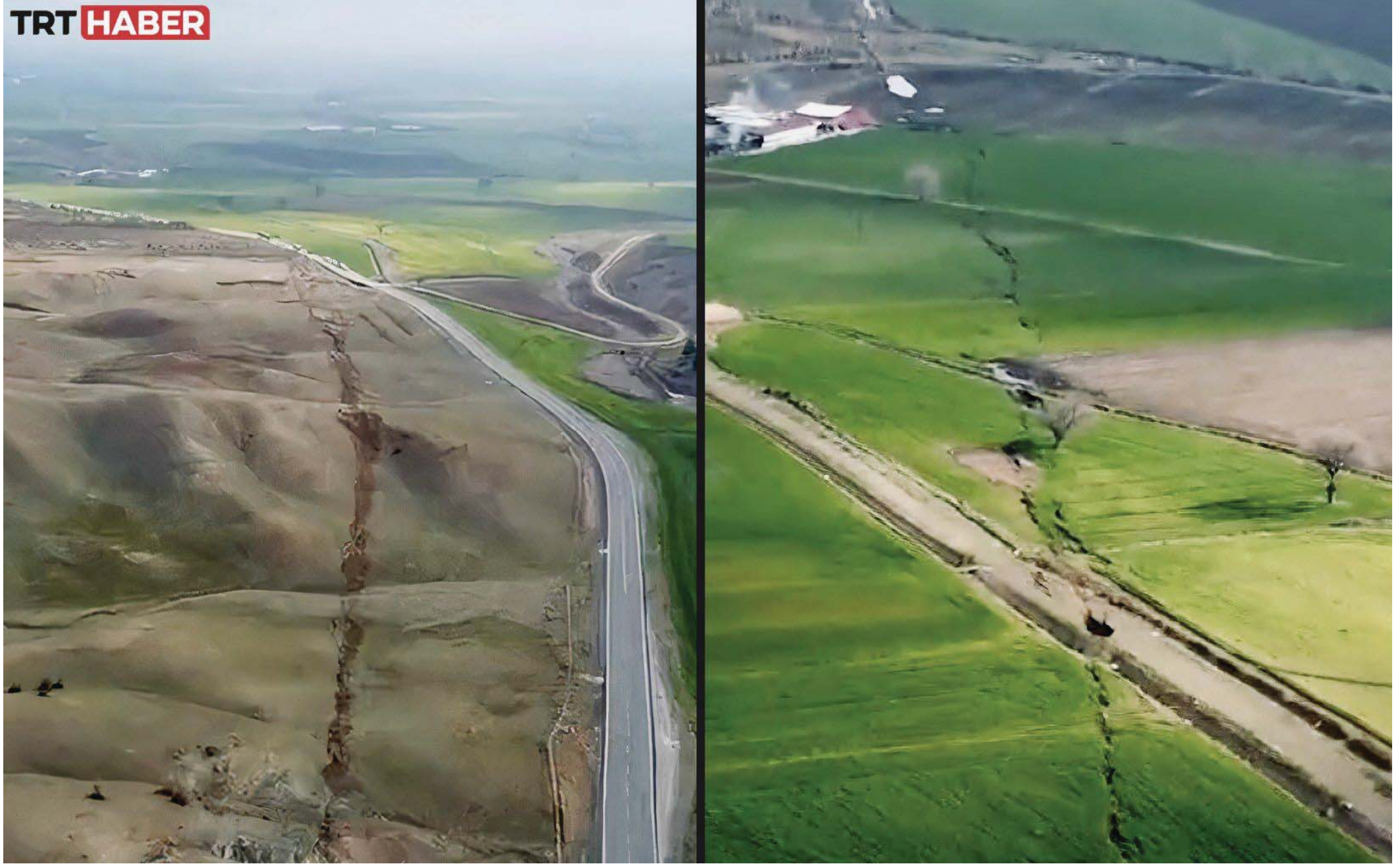
New aerial images show a tens of km long surface rupture associated with the M7.8 Turkey earthquake near Tevekkeli, Kahramanmaraş. Credit: @trthaber
