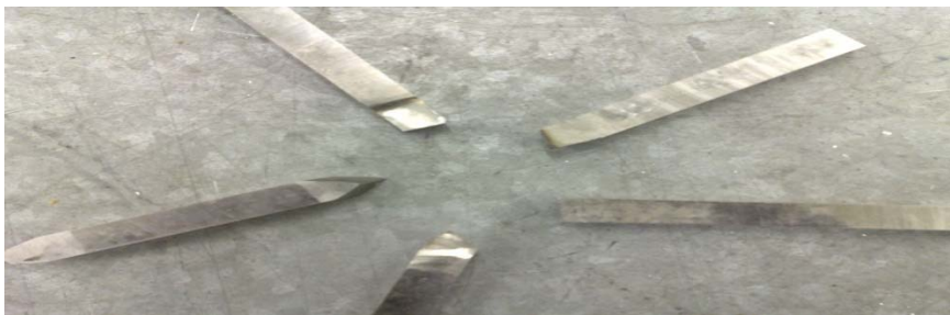
Figure3.10: Tools with side rake angle ( 5^\circ , 10^\circ , 15^\circ , 20^\circ , 25^\circ )
