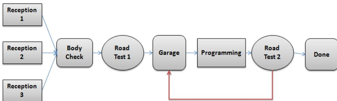
**Figure (5.1):** Processes flow chart for main repairing operation
