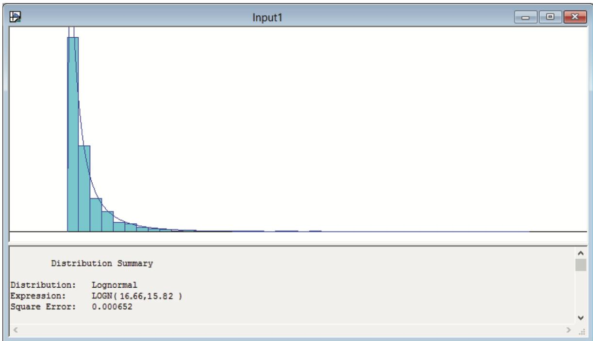
2. The graph below shows the distribution of maintenance stage calculated by input analyzer.
